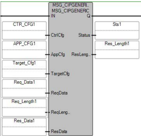
Figure 5 - CIP Generic Message Instruction for Run Mode Configuration Change
